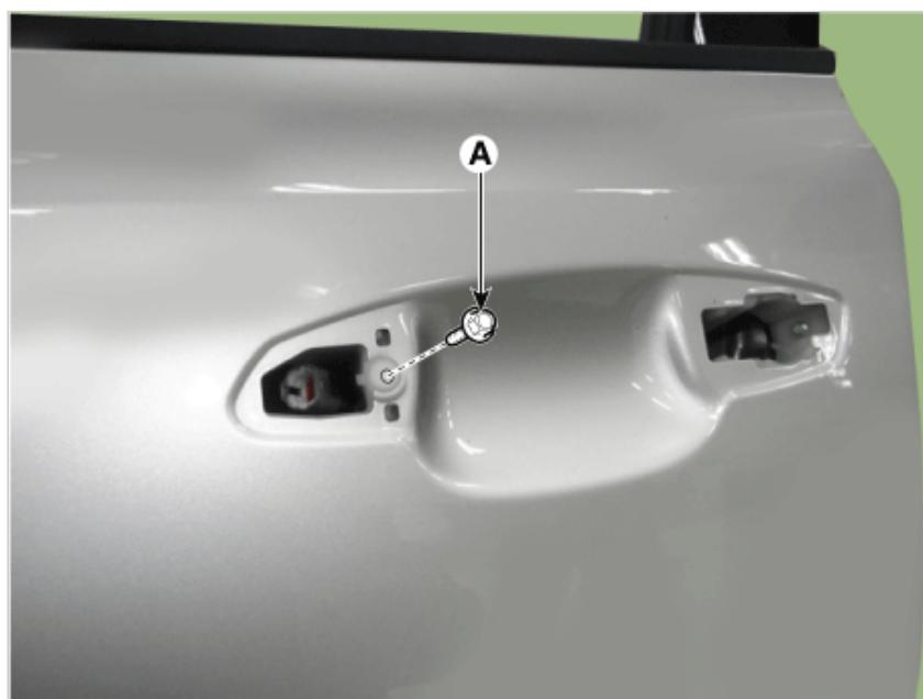
8. Disconnect the outside rear view mirror connector (A).
