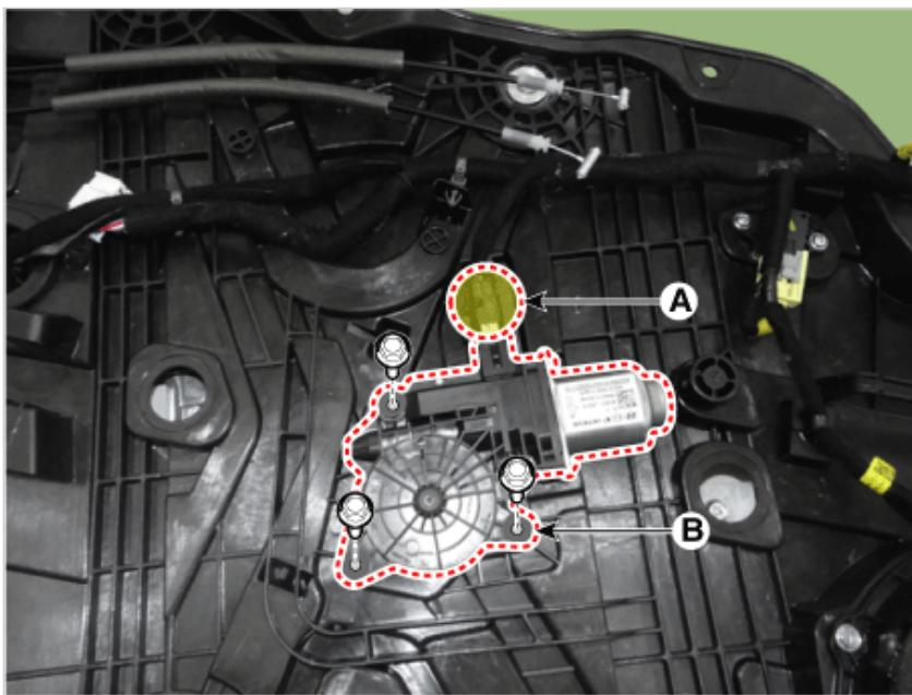
15. Disconnect the connectors and front door module wiring harness.
