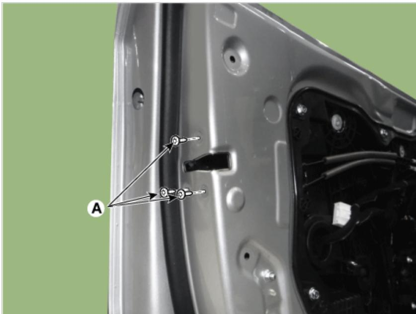
11. Remove the front door latch (A) after loosening the mounting bolts.
