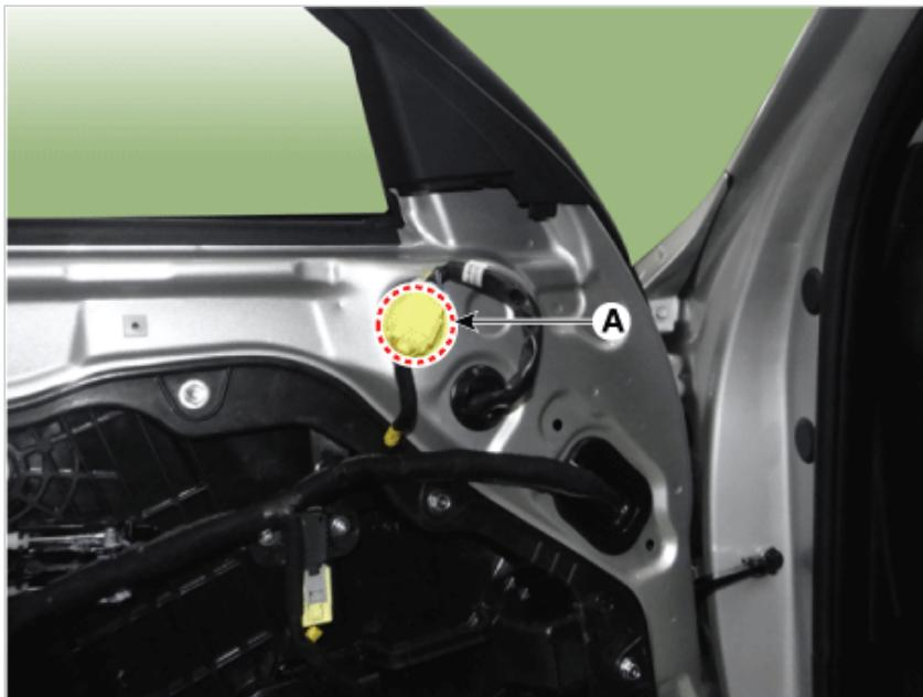
9. Disconnect the front door main wiring connector (A).
