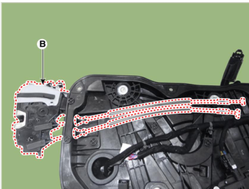
13. Remove the front door speaker (B) after disconnecting the connector (A).
